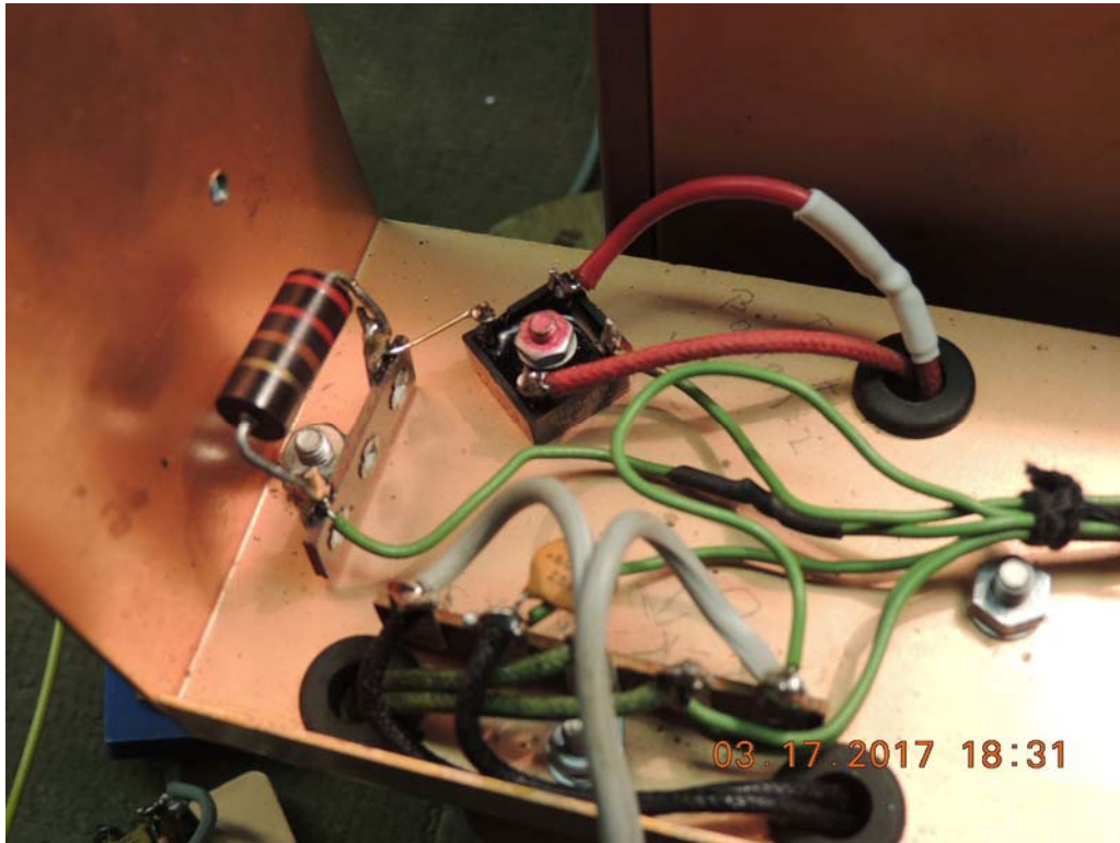
Power supply full wave rectifier upgrade
