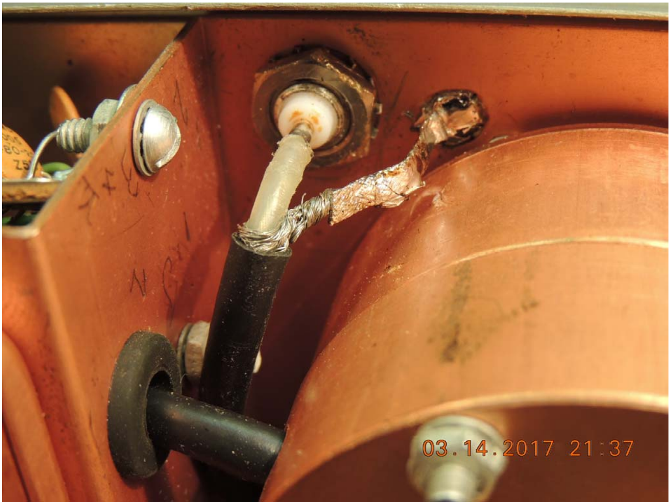
RF output BNC connector upgrade
