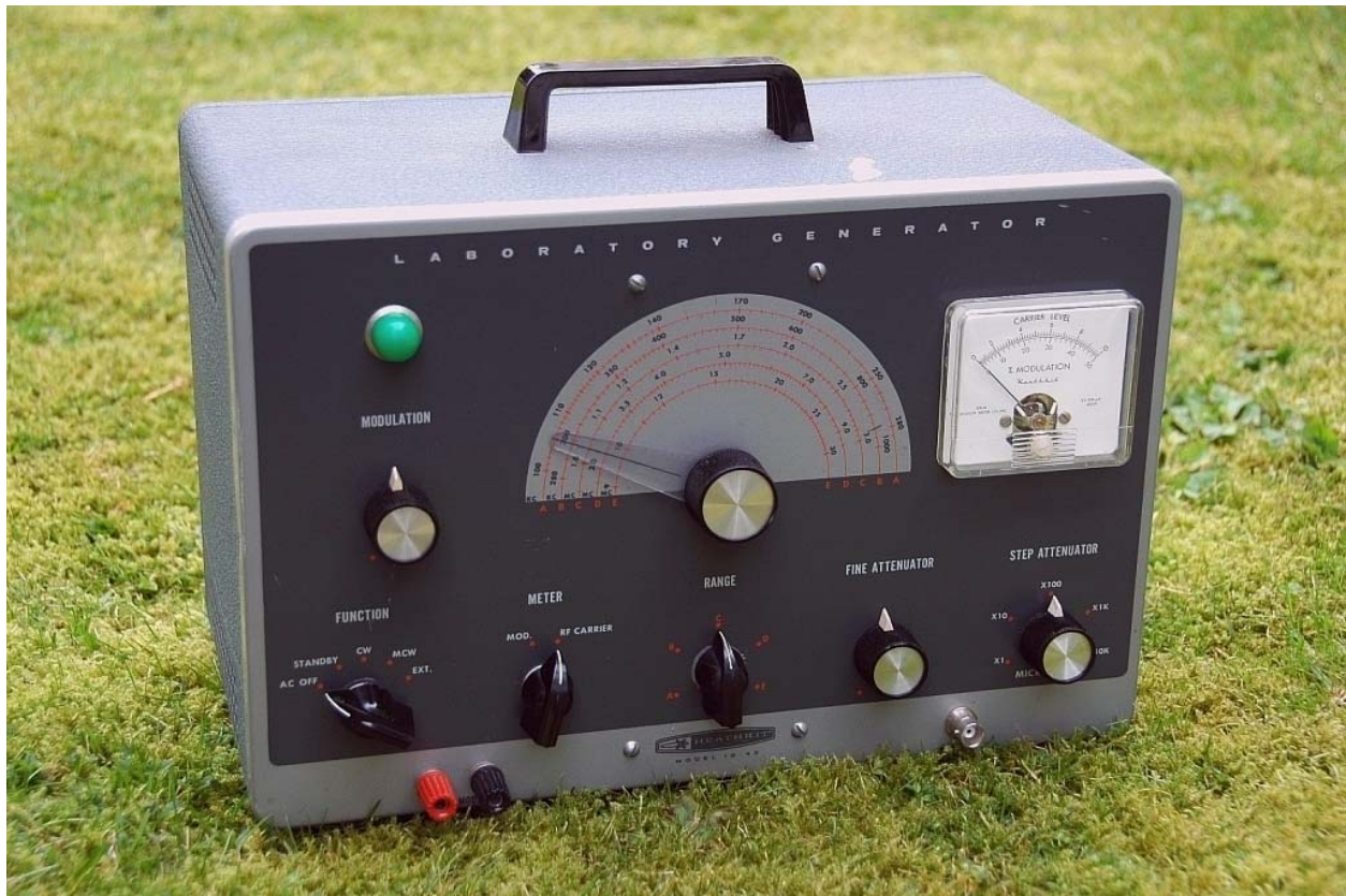
The IG-42 (note the chicken head knobs and BNC connector upgrade)
